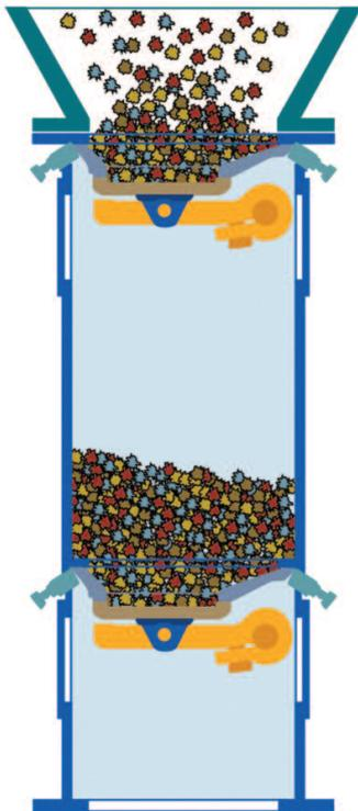
**d. Bottom gate opens, allowing material to pass on to downstream process**
